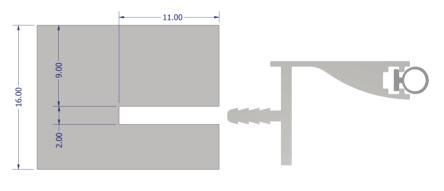
\* Note: Can be used on 16mm and 18mm board. Dimensions are still 9mm from top to top of cutout.
