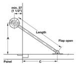
**Note:** Unscrew to increase and tighten screw to decrease braking effect.
